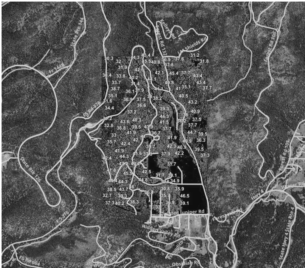
Figure 1. Canopy Height Model (CHM) of the Horseshoe Springs study area showing tree heights (green to red color gradient) overlaid on the terrain. Labeled points indicate maximum tree heights detected by the Lidar analysis. Roads (yellow lines) and stream courses (pink lines) are from Sandoval County databases.
